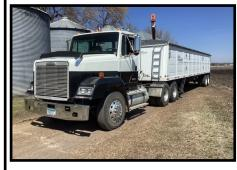
Detroit 60 series 11.1 Litre, 13 sd., air ride, 11.22.5 tires w/alum wheels, Alum Fuel Tank, twin screw, shows 389,623, which has been confirmed by ECM; 2011 MAURER 40' STEEL **HOPPER TRAILER, bought new, very** low miles, 24.5 tires, roll tarp, sight windows, very clean; 1976 FORD L800 TWINSCREW TRUCK w/20' Crysteel box & hoist
